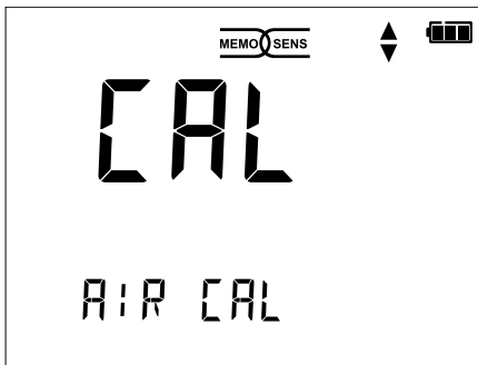
Oxygen calibration – step 1 (calibration in air)
