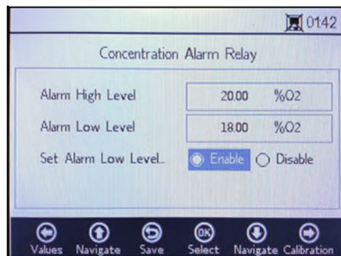
Figure 69. Analogues - Concentration alarm relay
