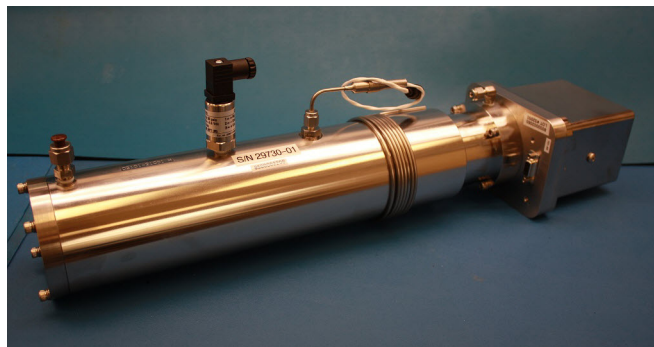
Figure B-11 New pressure sensor installed
