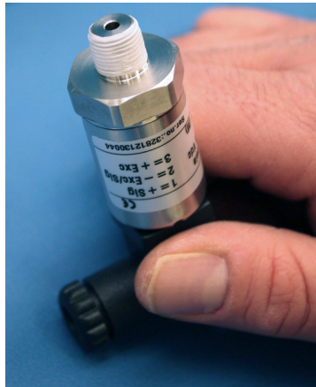
Figure B-15 Replacing seal tape
