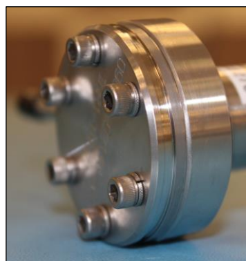
Figs 27 and 28. Stainless steel mirror marking: mirror with engraved X (left), mirror with grooved rim (right)
