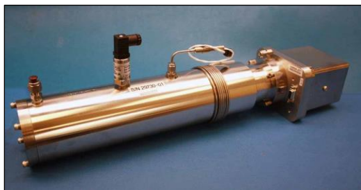
Fig 37. New pressure sensor installed.
