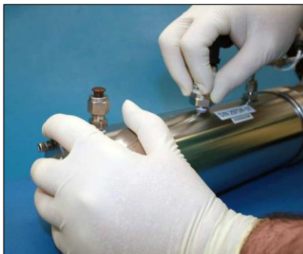
Fig 36. Replacing the pressure sensor
