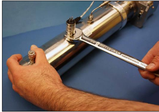
Fig 32. Removing the old pressure sensor
