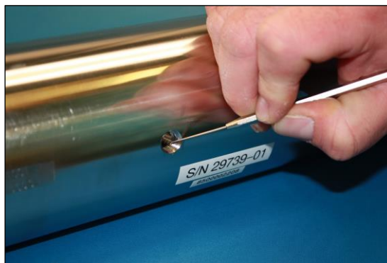
Fig 33. Removing excess seal tape from flange
