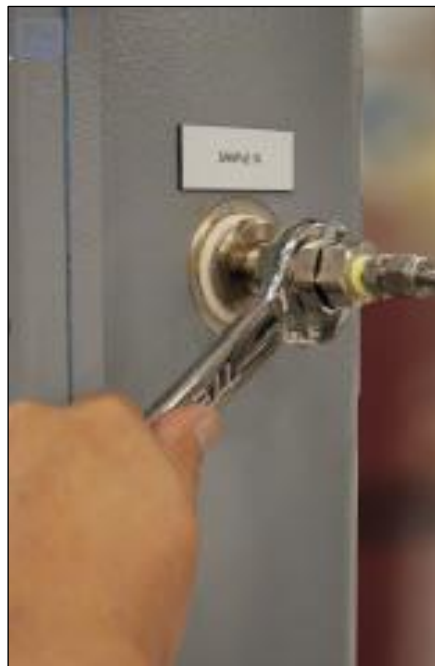
Fig 47. Removing the flame arrester
