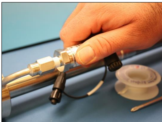
Fig 42. Replacing the pressure sensor.
