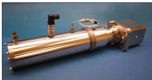
Fig 31. Removed measurement cell with pressure sensor oriented up
