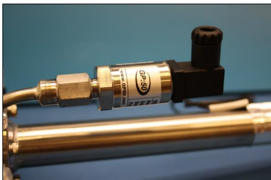
Fig 43. Newly installed pressure sensor positioning.
