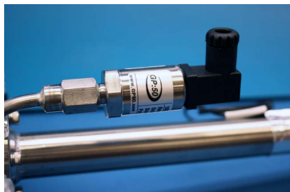
Figure B-10 Newly installed pressure sensor positioning
