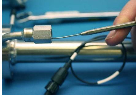
Figure B-7 Removing excess seal tape from flange
