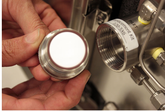
Figure B-12 Inspecting the membrane separator filter
