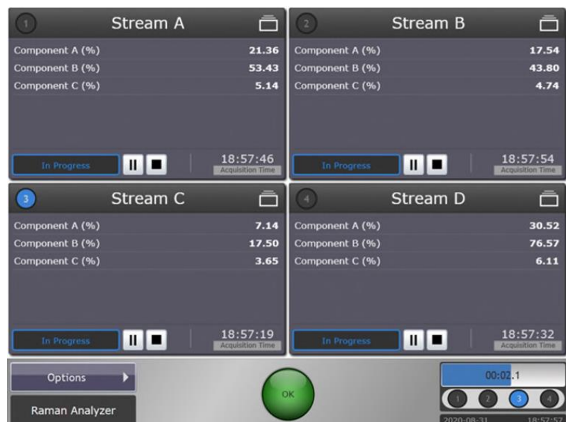
Figure 5. Raman RunTime's main view in a Raman Rxn four channel analyzer
