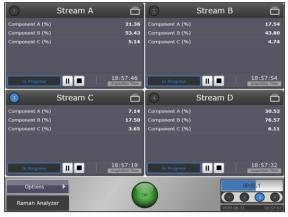
Figure 38. Raman RunTime main screen for a Raman Rxn4 four channel analyzer
