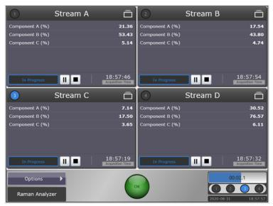
Figure 4. Raman RunTime's main view in a Raman Rxn four channel analyzer
