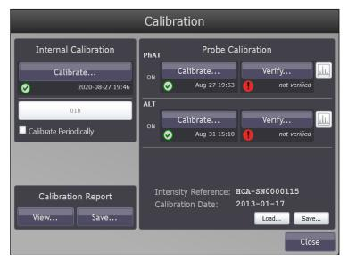
Figure 47. Calibration window for a Raman Rxn Hybrid analyzer
