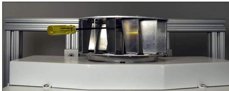
Figure 14. Top-mounted fan impeller with shroud removed
