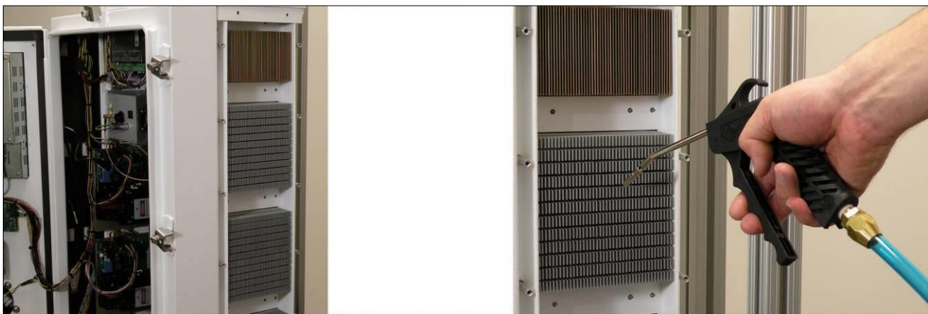
Figure 111. Cleaning heat sinks with compressed air or water
