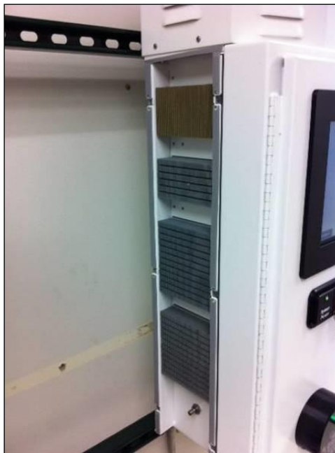
Figure 12. Heat sinks on the side of the Raman Rxn5
