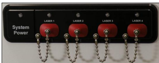
Figure 45. Switch indicator panel
