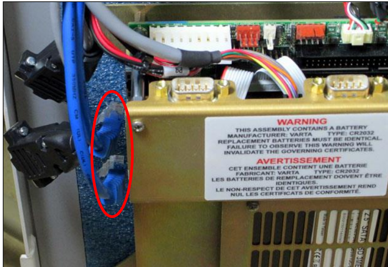
Figure 133. Remove RJ45 cables
