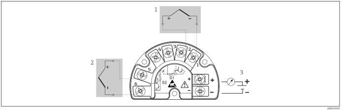
🖻 6 Wiring of the field transmitter, RTD, dual sensor input
