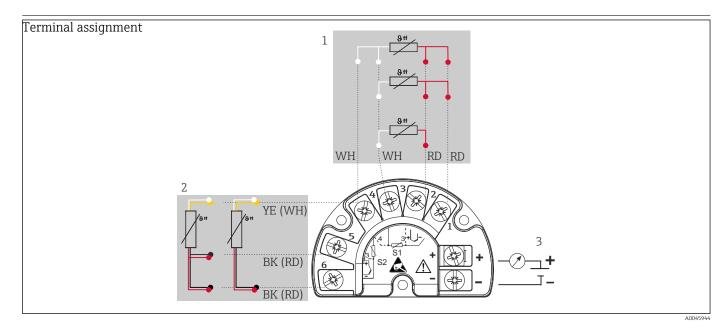
🖻 17 Wiring of the field transmitter, RTD, dual sensor input
