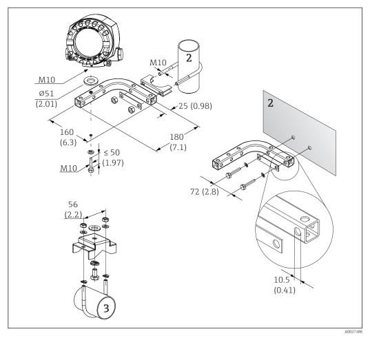
Installation of the field transmitter using the mounting bracket, see chapter 'Accessories'. Dimensions in mm (in)
