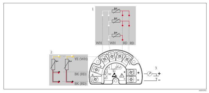
🖻 5 Wiring of the field transmitter, RTD, dual sensor input
