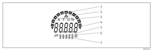
■ 15 LC display of the field transmitter (illuminated, can be plugged in in 90° stages)
