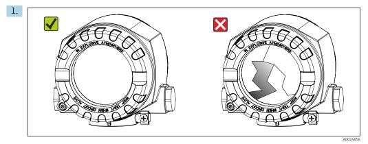
Unpack the temperature transmitter carefully. Is the packaging or content damaged?
