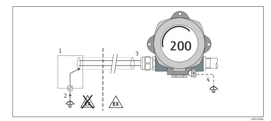
■ 10 Shielding and grounding the signal cable at one end with HART<sup>®</sup> communication
