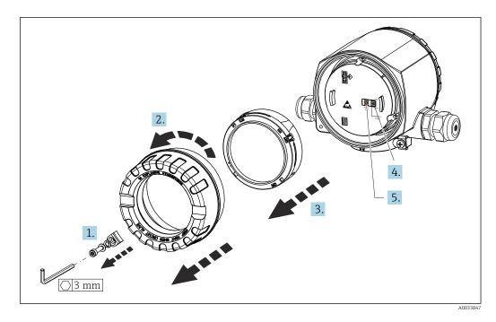
Procedure for setting the DIP switch or activating the proof test:
