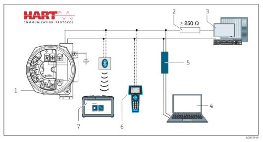
9 HART<sup>®</sup> connection with other power supply units that do not have a built-in HART<sup>®</sup> communication resistor
