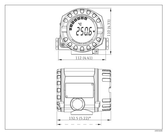
20 Die-cast aluminum housing for general applications, or optional stainless steel housing (316L)
