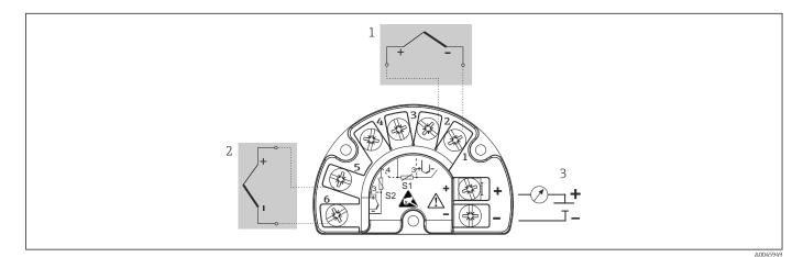
🖻 18 Wiring of the field transmitter, RTD, dual sensor input
