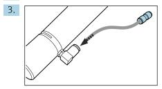
Connect the hose of the compressed air supply at the installation location to the opening of the elbow plug.
