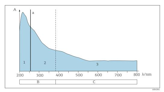
Ranges of parameters in the absorption spectrum
