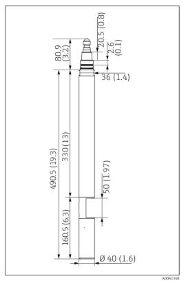
Dimensions of spectrometer with
