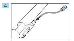
Connect the hose of the compressed air supply to the opening of the elbow plug.
