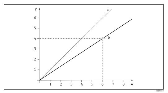
23 Principle of a 1-point calibration
