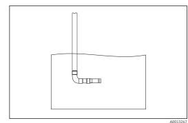
I1 CYA112 immersion assembly and CYH112 holder installed horizontally, fixed installation
