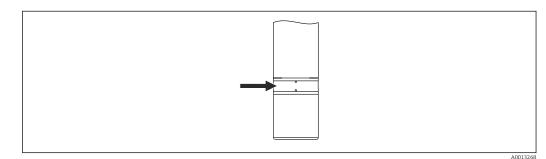
Image: Alignment, arrow points in the flow direction
