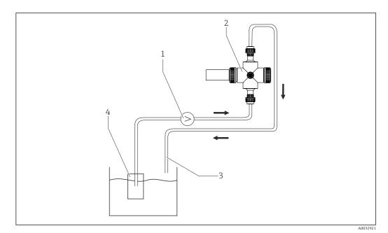
■ 10 Connection diagram with open outlet, arrow points in the flow direction
