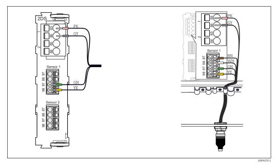
■ 17 Spectrometer connection to input (left) or via M12 plug (right)
