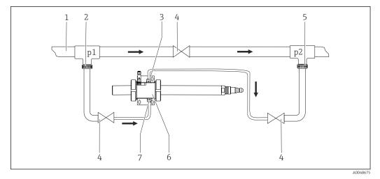
☑ 14 Connection diagram with bypass
