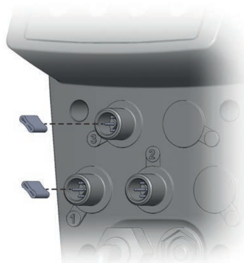
Fig. 16: Conductive rubber hoses in the connections 1 and 3 of the MAGDOS LA/LD
